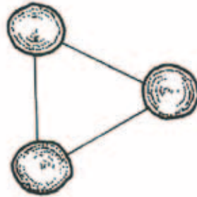
Fig 68: Where three limbs/stems are to be connected, a triangular connection has to be installed to reduce swaying in all directions (ZTV-Baumpflege 2006).
